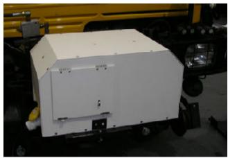
components. This results in a light weight & efficient unit. A mounting bracket is provided to position the DG4000 on the front mounting Schmidt plate (front mounting plate conforming to DIN 76060 size 3 code D11) as supplied by Mercedes Benz.
